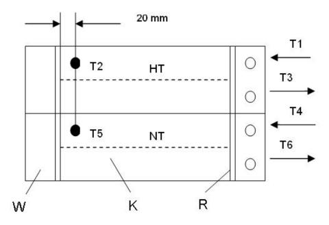
Positions of temperature measuring points (T1 to T6)
